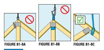
**NOTICE** Do not lift single Trusses by the Webs as shown in Figure B1-8B, as this will cause Lateral Bending in the Truss and damage to the Truss Plates and web member.
