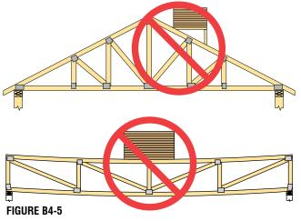
DO distribute Loads over as many Trusses as possible. Position stacks of materials flat with the longest dimension perpendicular to the Trusses as shown.
