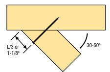
FIGURE B8-10 Corner jack to corner Girder Truss
