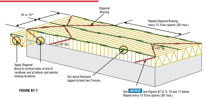
\*Spacing between rows of Top Chord Temporary Lateral Restraint (TCTLR) shall be 10' o.c. max. for 3x2 chords and 15' o.c. for 4x2 chords.
