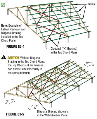
Note: The Purlins alone will not adequately brace or prevent buckling of the Top Chord and must themselves be braced. This bracing can be provided in a number of ways including:
