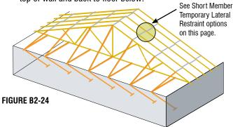
**NOTICE** The following three Short Member Temporary Lateral Restraint Options require that the **Diagonal Bracing be installed continuously**. Install Diagonal Bracing to the Top Chord plane immediately after the intial five Trusses have been set and restrained. Thereafter, install Diagonal Bracing to each subsequent set of four Trusses.
