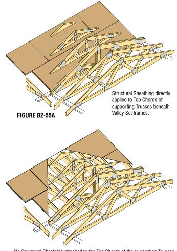
No Structural Sheathing attached to the Top Chords of the supporting Trusses beneath the Valley Set frames. The on-center spacing of the Valley Set frames, as measured along the slope of the Top Chord of the supporting Trusses, must be less than or equal to the maximum Purlin spacing specified on the TDD for the Top Chord of the supporting Trusses. Add Diagonal Bracing to the Top Chord Plane of the supporting Trusses if the Valley Set frames are  $\geq$  20' in length.
