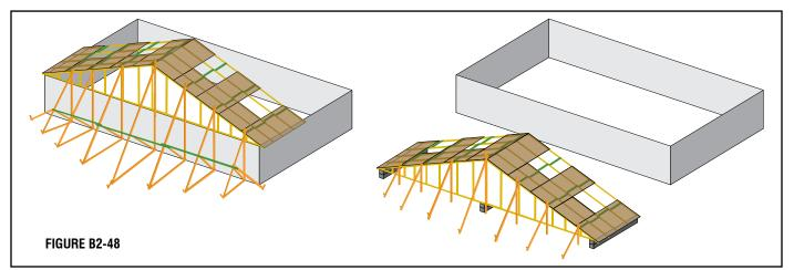
Keep Trusses Straight Durina Hoistina: Lona Span Trusses are very prone to bending out-ofplane while being lifted into place. It is very important to provide support so the Trusses flex as little as possible. A good hoisting device and Spreader Bar can provide support and be a real time saver.
