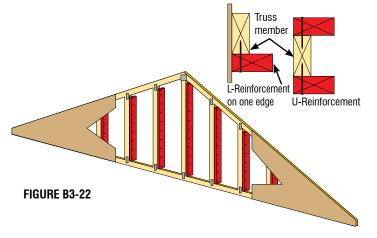
Scab Reinforcement is installed on one face of the Web. It is often more structurally efficient for multiple-ply Webs and provides easier nailing because it is applied to a wide-face of the Web.
