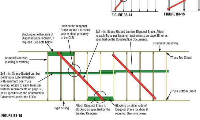
**Note:** To help transfer large Bracing forces into the roof and ceiling Diaphragms, dimension lumber Blocking may need to be installed between the Trusses on either side of the Diagonal Brace location as shown in Figure B3-16. Cut the Blocking to fit snuggly between the Trusses and attach to the Trusses and the Diaphragm. The Blocking helps to transfer the lateral Load directly from the Diagonal Brace into the Diaphragm.
