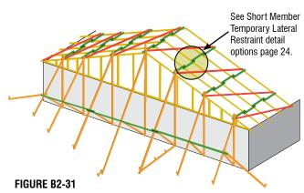
Example of Diagonal Bracing on first five Trusses with Ground Bracing to top of Building wall and back to floor below:
