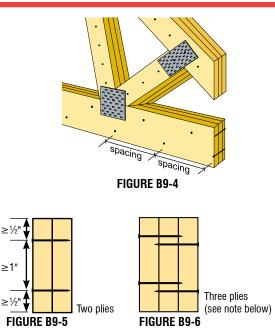
Girder Trusses of up to three (3) plies are permitted to be fastened together with nails. Nail each additional ply in accordance with the specified schedule found on the TDD.
