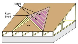
For conventionally framed dormers, as shown in this figure, the Top chords of the supporting Trusses beneath the dormer must be restrained and Braced with Structural Sheathing, as shown, or with rows of Lateral Restraint and Diagonal Bracing, to prevent buckling under Load. See NOTE below for assumed flow of Loads to Trusses depending on the method used to frame a valley.
