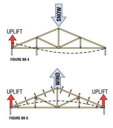
✓ Wind and seismic forces acting on the Building produce lateral Loads that are often transferred at the Truss bearing locations. The magnitude and direction of these wind and seismic Loads are to be provided by the Building Designer.
