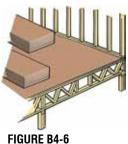
ODN'T drop Loads of any materials on Trusses. Truss damage from the impact is possible even if the weight of the material is small.
