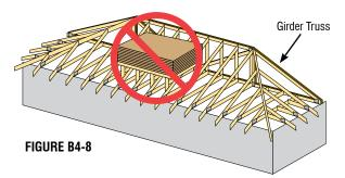
**DON'T** stack materials at locations that will produce instability, such as on cantilevers, overhangs or near Truss-to-Girder Truss Connections.
