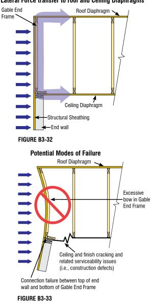
✓ Typical Gable End Frame Bracing/reinforcement details include Blocking at the ceiling and roof level Diaphragms, gable stud reinforcement, horizontal reinforcement and/or Diagonal Bracing, mechanical Connectors/straps and specific fastener size and frequency schedules.
