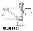
DO NOT attach the deck ledger to 2x\_ ribbon board unless a special detail has been provided by the Truss Designer or Building Designer.
