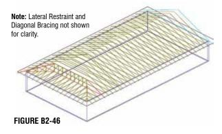
DON'T stack materials or stand at locations that will produce instability, such as on cantilevers, overhangs, end jacks or near Truss-to-Girder Truss Connections.
