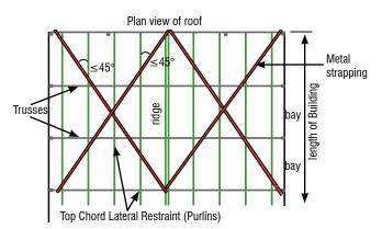
**Note:** Metal strap cross Bracing is typically used when Purlins are mounted flush between Trusses. Run Bracing to the fourth Truss on 48' and wider buildings.
