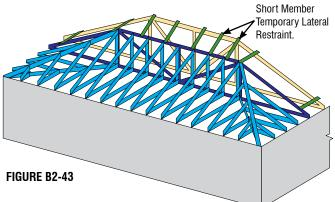
Step 4: Install remaining Hip Trusses. For the flat portion of each Hip Truss, use Short Member Temporary Lateral Restraints that are at least double the length of the first set of Short Member Temporary Lateral Restraints. For the sloped chords of the Trusses, install Short Member Temporary Lateral Restraints according to one of the three options on page 24.
