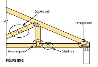
Describe the damage directly on the original Truss Design Drawing (TDD) included in the JOBSITE PACKAGE.
