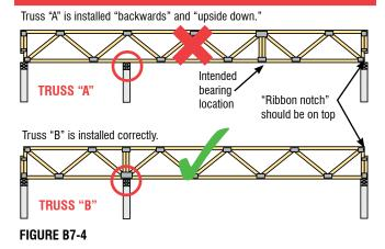
✓ It is critically important that Bottom Chord Bearing PCT be installed with the correct side up and in the correct orientation. Many Truss Manufacturers will use supplemental tags (as shown below) to instruct and warn the Contractor to correctly position Trusses during erection/installation.
