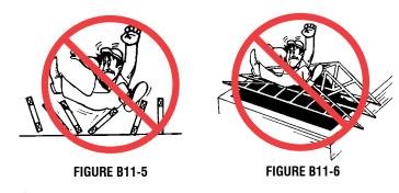
▲ **DANGER** Do not stand on Truss overhangs until Structural Sheathing has been applied to the Truss and overhangs.
