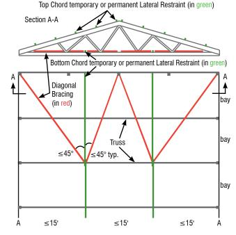
FIGURE B10-19 Bottom Chord Restraint and Bracing
