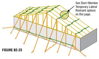
Example of first five Trusses with Interior Ground Bracing to top of wall and back to floor below:
