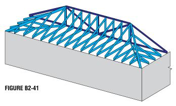
Alternate Option to Step 1 & 2: Assemble the Girder Truss and jacks on the ground and lift the entire assembly into place. Be sure to get guidance from a Registered Design Professional to ensure modules are designed and installed safely and properly (see page 29 for information on an alternative installation method).
