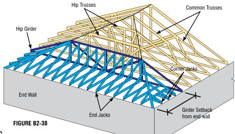
Step 2: Install all remaining corner and end jacks with all permanent Truss-to-bearing Connections (e.g., hangers, clips and tie-downs).
