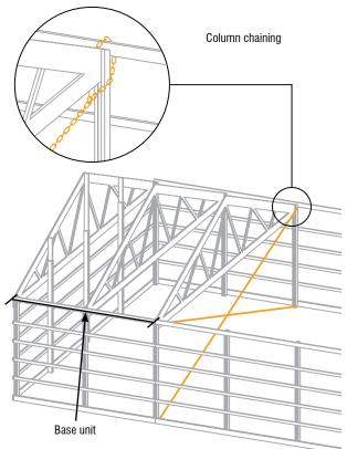
Purlins, Truss Web Restraint/Bracing & some nailers omitted for clarity. See Step 3 for Temporary Restraint & Bracing requirements for the Trusses.
