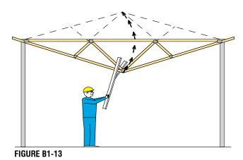
Trusses with spans less than or equal to 30' should be raised into position by lifting at Top Chord joints nearest the guarter points of the span.
