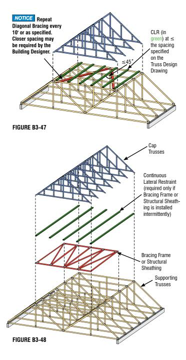
✓ The supporting Trusses shall have all of the required Temporary Bracing discussed in BCSI-B2 and Top Chord Permanent Bracing discussed here installed BEFORE installing the cap Trusses.
