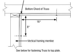
FIGURE B8-15 Floating gypsum corner (Truss perpendicular to wall)
