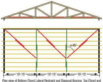
Plan view of Bottom Chord Lateral Restraint and Diagonal Bracing. Top Chord an Web Lateral Restraint and Diagonal Bracing not shown for clarity.
