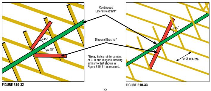
✓ For Webs that require two rows of CLR, the concepts are the same as those used to brace a single row of CLR (see Figure B10-34 and B10-35 for examples). Position the Diagonal Brace(s) to cross the Webs in close proximity to each row of Lateral Restraint to minimize the out-of-plane bending forces in the Web. Attach the Diagonal Brace(s) as close as possible to the Top and Bottom Chord Plane and to each Web that the Diagonal Brace(es) crosses.
