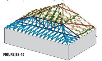
✓ If there is a hip at one end of the Building and a gable at the other, a good practice is to start the Truss installation at the hip end.
