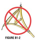
✓ Due to treatment effects, fire retardant treated Trusses require special care when handling to prevent chord and web member breakage. Limit exposure to the elements per manufacturer's recommendations.
