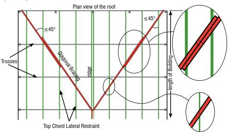
**Note:** Diagonal Braces run to the fourth Truss on 48' & wider buildings. Braces lap two rows of Lateral Restraint if Diagonal Brace is spliced. Use 2-16d (0.135x3.5") nails at each Diagonal Brace-to-purlin Connection.
