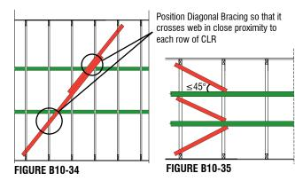
**Note:** Splice reinforcement, similar to that shown in Figure B10-31 on page 83, may also be used with Diagonal Bracing in lieu of overlap shown here.
