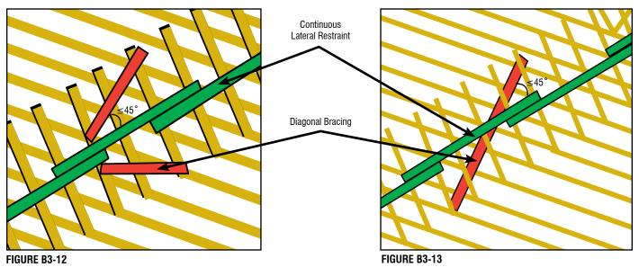
For webs that require two rows of CLR, the concepts are the same as those used to brace a single row of CLR (see Figure B3-14 and B3-15 for examples). Position the Diagonal Brace(s) to cross the webs in close proximity to each Lateral Restraint to minimize the out-of-plane bending forces in the web. Attach the Diagonal Brace(s) as close as possible to the Top and Bottom Chord Plane and to each web that the Diagonal Brace(s) crosses.
