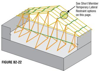
Example of first five Trusses with Exterior Ground Bracing:
