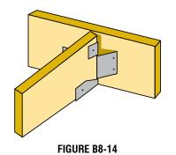
Some Building codes specify Connection requirements between the Truss and the bearing surface. It is imperative that the installer be familiar with the requirements that apply for each job.
