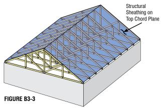
☑ Wood or metal Purlins are most often used in applications where Trusses are spaced greater than 4' o.c. The Purlins must be properly sized and fastened to the Top Chord of the Trusses in accordance with the specifications found in the Construction Documents. The Trusses must be designed so that the maximum allowable unbraced length for the Top Chord is greater than or equal to the on-center spacing of the Purlins.
