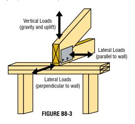
✓ Wind Loads acting on a Truss, as well as certain multi-span Truss applications supporting gravity Loads, can produce uplift reactions at Truss bearing locations. The magnitudes of these uplift reactions are typically provided on the Truss Design Drawing (TDD).
