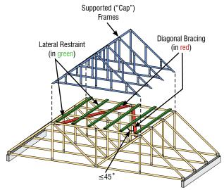
Note: Some Lateral Restraint and Diagonal Bracing not shown for clarity. FIGURE B2-52
