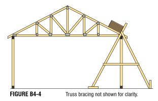
ODN'T stack materials at or near the midspan of the Trusses. Never exceed stack heights per Table B4-1, page 53, unless alternative information is provided by the Building Designer, Truss Designer or Truss Manufacturer.
