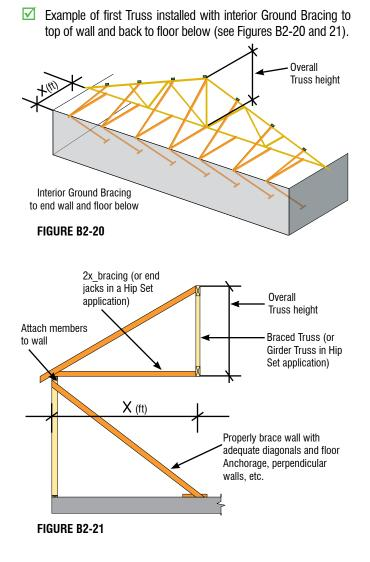
✓ X = wall setback (ft) = overall Truss height (ft-in) rounded to next full Truss Spacing (ft), or Girder Truss set back in hip end framing. For example, if the overall Truss height is 5'-6" and the Trusses are to be spaced at 2' on-center (o.c.), use a wall setback, X, of 6' (i.e., three Truss Spaces @ 2' = 6' > 5'-6").
